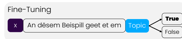
(a) The model is fine-tuned on detecting whether a topic is present in a sample x or not (= binary classifier). Translation: This example is about...
