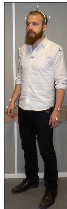
Figure 3: Each subject wears markers on hands, wrists, elbows, shoulders, sternum, and three markers mounted on a head-worn tiara.
