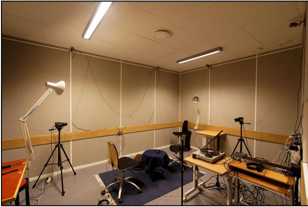
Figure 1: The recording studio. Video cameras are on tripods to the left and right in the picture. The turntable used for synchronization is visible just right of center, with the B&K microphones in microphone stands on either side. Motion capture cameras are barely visible, mounted along the walls just under the ceiling.
