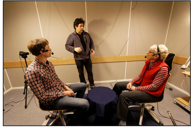
Figure 2: The recording studio during the instruction phase of a session. Subjects are wearing headmounted microphones and head bands with Optitrack markers, and additional markers are fixed to torsos, arms and hands.
