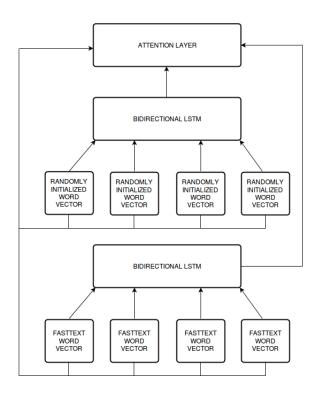
Figure 2: Multi-Channel LSTM architecture
